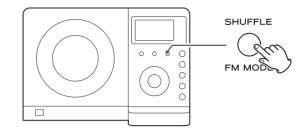
During playback, press the SHUFFLE button to change the shuffle mode.
